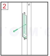
to tighten the electromagnet
